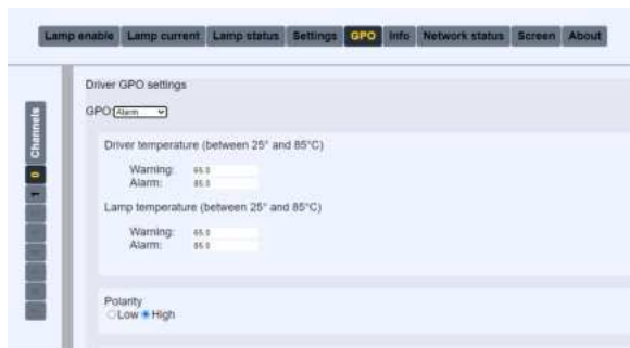
Pic. 52. GPO - Alarm
