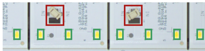
Detection of misplaced and rotated SMD connectors
